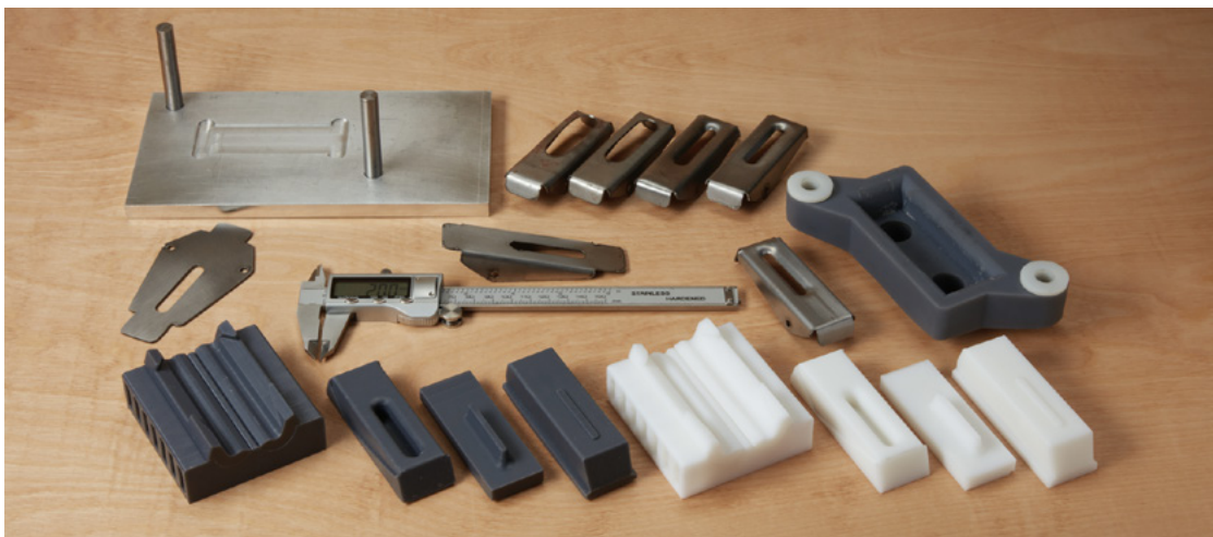
Printed dies and metal parts iterations for forming the blade guard.
