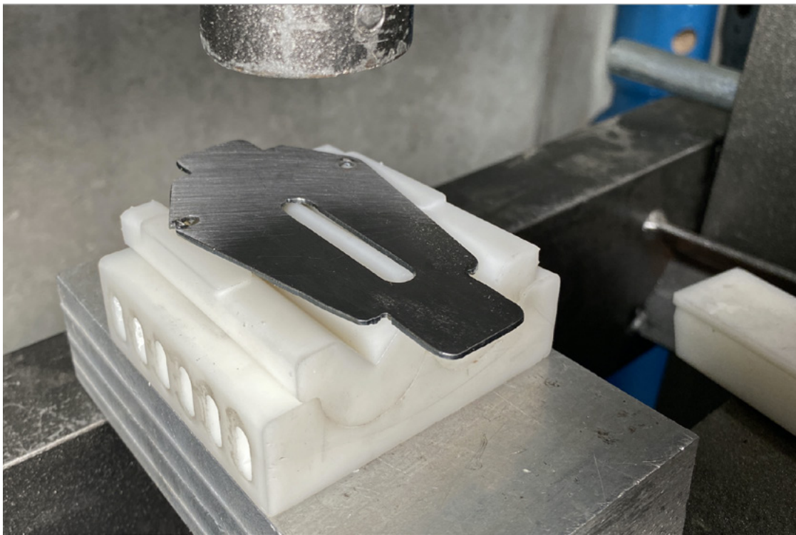
The pressing operation for bending the flanges.
