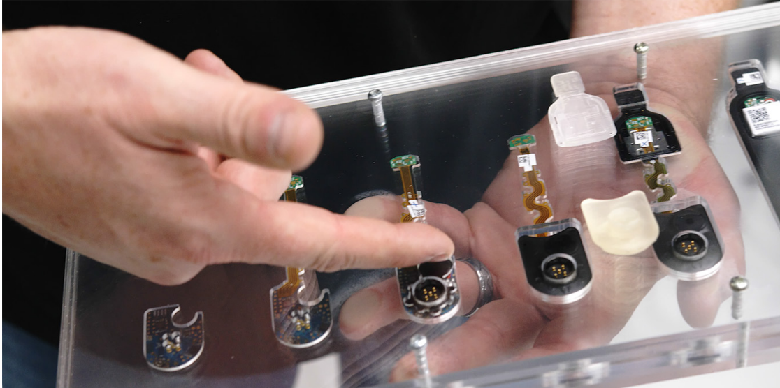
Google's ATAP team used 3D printed stand-ins , or surrogate parts instead of overmolded electronic sub-assemblies for the initial tool tuning at the factory
